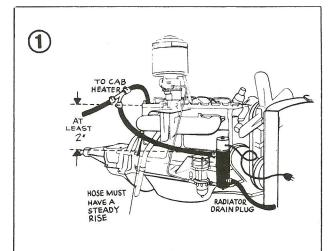
Engine Heater connected to draw water from radiator drain petcock and to inject it into engine through cab heater hose using "T" connection.
