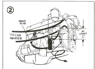
Take the cold water from the motor drain plug and inject the hot water into the hose line going to the water pump.
