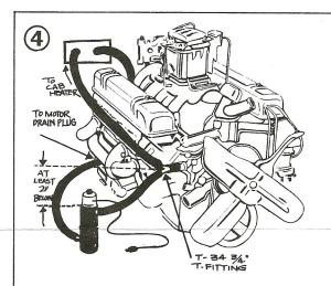
Engine Heater connected to draw water from the motor block drain plug and to inject it into the engine through the cab heater hose using "T" connection.
